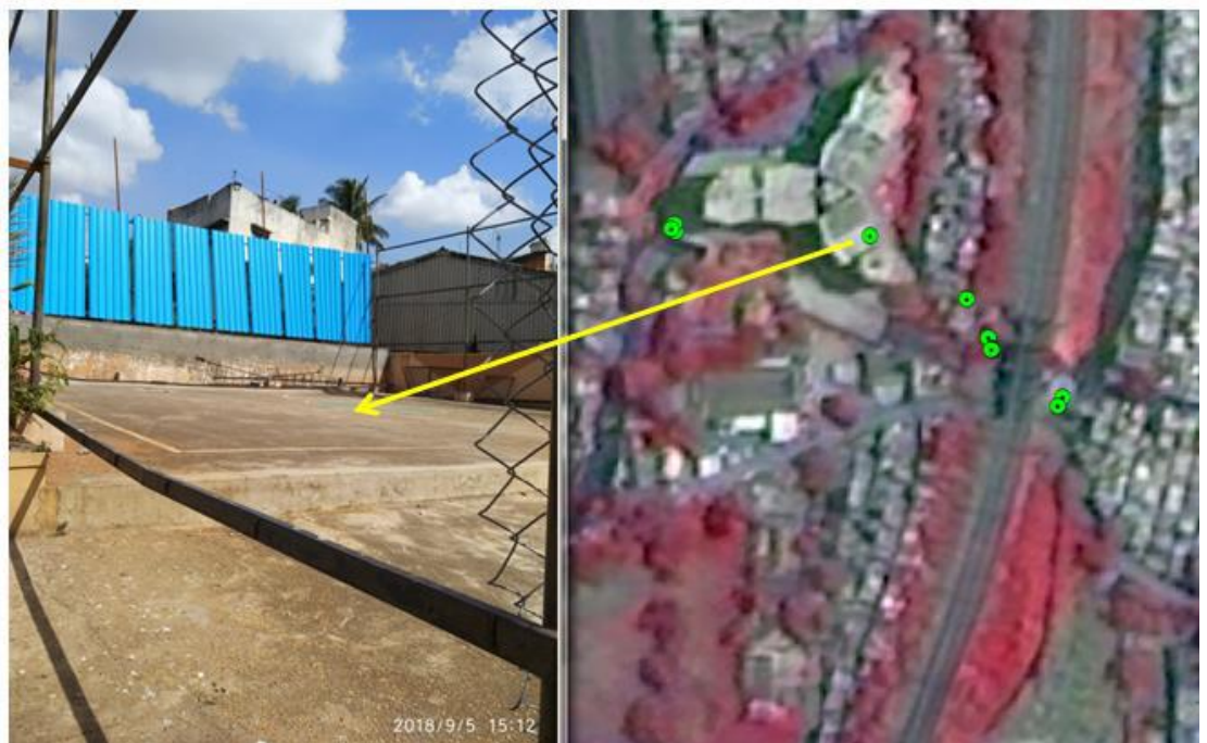
Drain encroached and covered by an apartment
